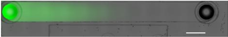
Figure 7. A merged fluorescence and bright field image of channel slide in a solute-gradient condition. FITC-PBS solution was used to visualize the gradient situation. Scale bar is 5 mm.
