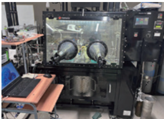
Fig. 1-1 An argon glove box with purification system.
