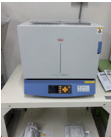
Fig. 1-2 A box-type electric furnace.
