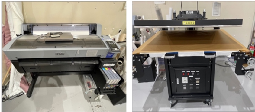
Fig. 2. Inkjet printer for sublimation transfer (left) and thermal transfer device (right).
