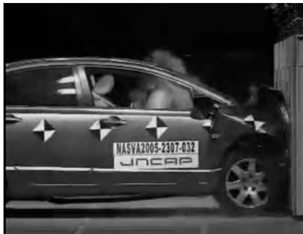
Figure 5.2 A picture showing full-lap frontal collision test according to J-NCAP (Japan New Car Assessment Program) for a passenger car (1800cc class sedan) [1].
