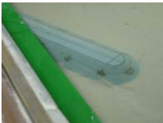
Photo 3 Hydraulic model of “Kami-Naizen”; s=1/100
