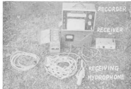
Fig. 4. General view of the deck unit (receiving hydrophone, demodulator and recorder).
