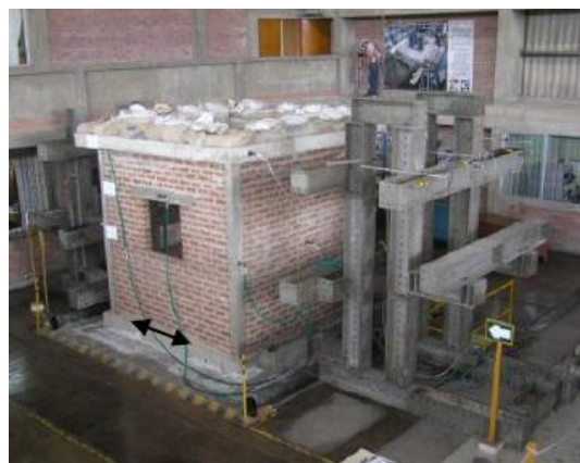
Figure 56 – Model Structure for Shaking Table Test of Confined Masonry Brick-Walls Construction with Additional Reinforcement (Minowa, et al., 2010)
