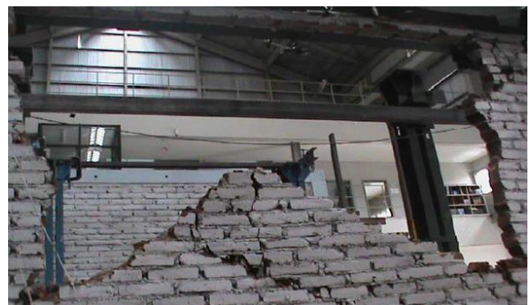
Figure 47 – Cracks Pattern of Second Brick-Wall Panel with Low Quality of Bricks (Research Institute for Human Settlements & JICA, 2012)
