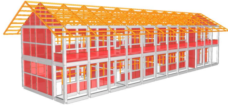
Figure 81 – 3D Model of Two Stories School Building with Confinement
