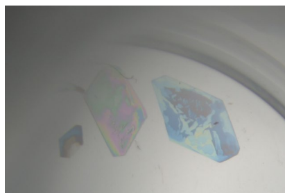
Figure S8. Morphology of single crystals of AP-monomer obtained by slowly evaporating ethyl acetate into its ethanol solution.
