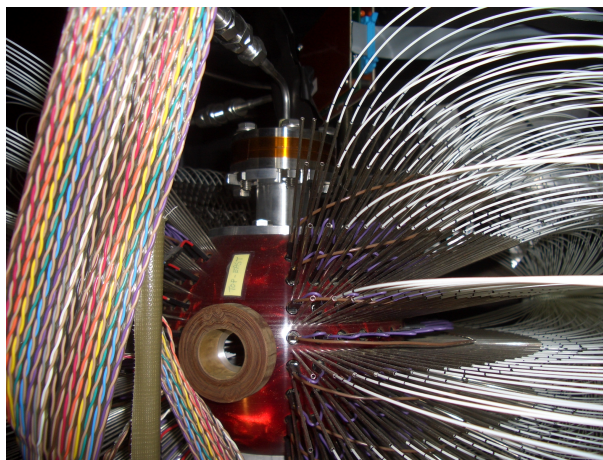
Figure 2.25: Bowling ball for the gain monitoring system. The central red ball contains the liquid dye. Many white thin fibers are secondary quartz fibers.
