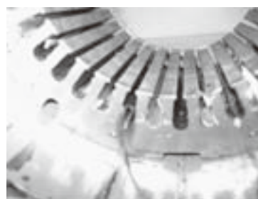
Fig. 1 Photograph of DI-BSCCO® (Type ACT) short sample in a slot of stator core.
