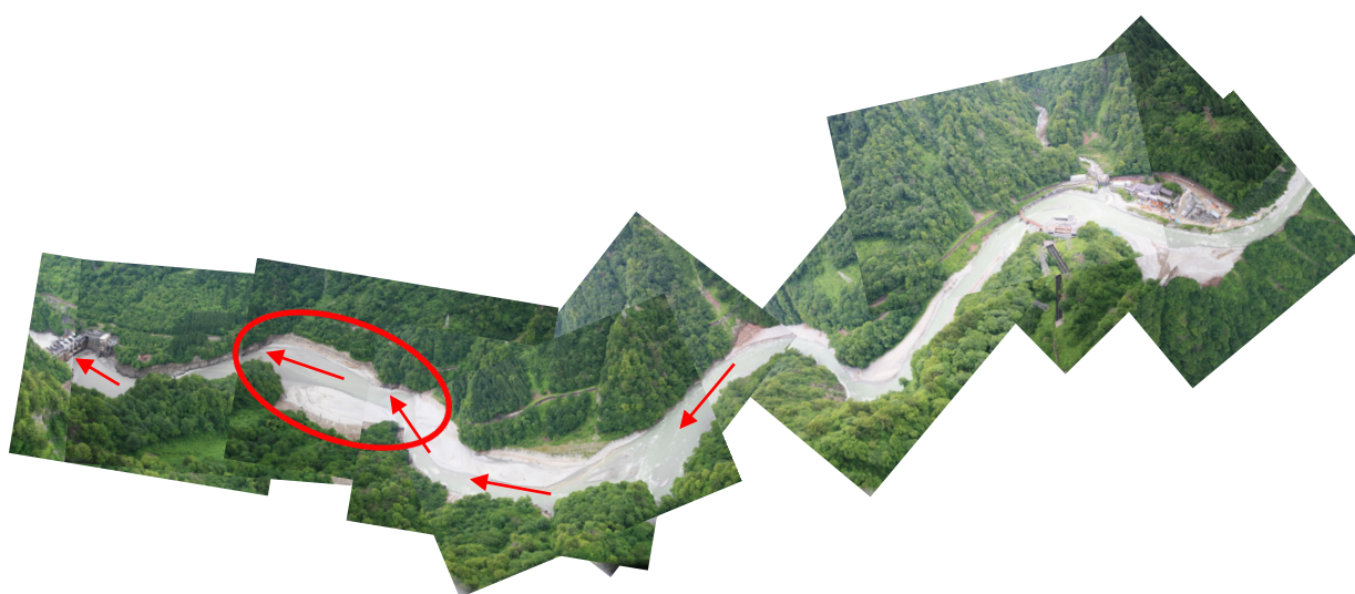
Figure 1.6 Developed flushing channel during 2012 free-flow flushing operation in Dashidaira reservoir (Photo from Kurobe River Work Office); Red arrows show the flow direction and red oval illustrate the wide area of the reservoir with a dead zone along the left bank.
