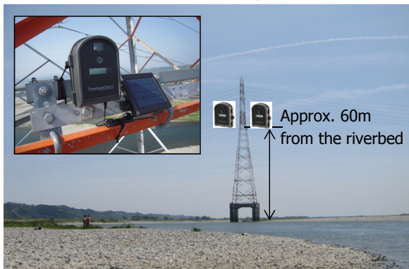
(b) Interval-recording-cameras were located in a middle of the river channel, approximately 60 m high from the riverbed. These cameras have been equipped with solar panels, enabling data accumulation of a longer period.
