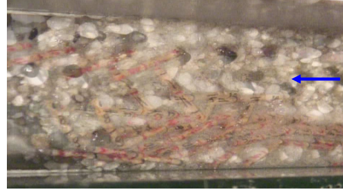
Fig. 15 Flow motion of driftwood at forefront of debris flow
