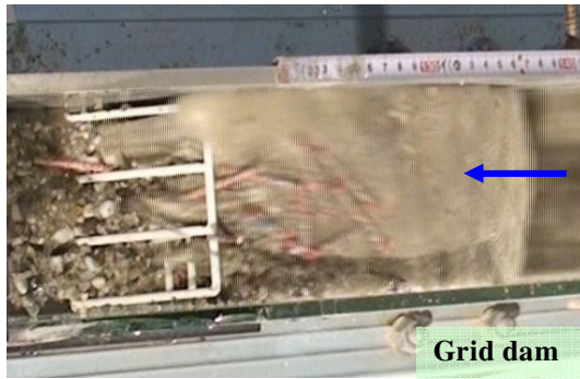
Fig. 16 Flow motion of driftwood at upstream of check dams
