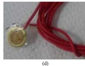
Fig. 2. Schemas of a conventional piezoelectric device and a novel piezoelectric transducer. A conventional piezoelectric device (a), a skin-mediated piezoelectric transducer (SPT) (b), and the detailed composition (c) and photograph (d) of an SPT.
