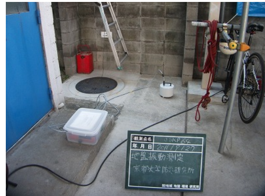
Photo 1 Microtremor observation at a strong motion station in the Osaka sedimentary basin
