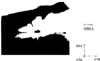
Fig.2-10 Bright field cross-sectional TEM image of 2ML-thick InAs.
