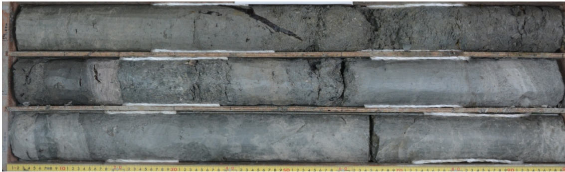
Photo 5 Example of boring core (depth 159m-162m).
