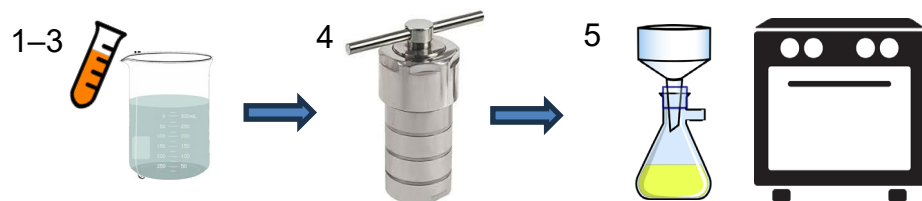
Preparation of BPO-zeolite composites by hydrothermal treatment
