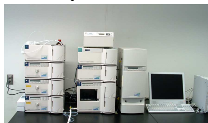
図 5 GC-MS (Trace DSQ、Thermo Quest)
