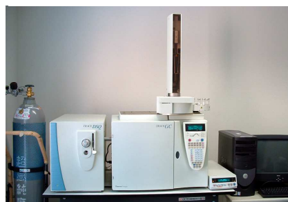
図 5 GC-MS (Trace DSQ、Thermo Quest)
