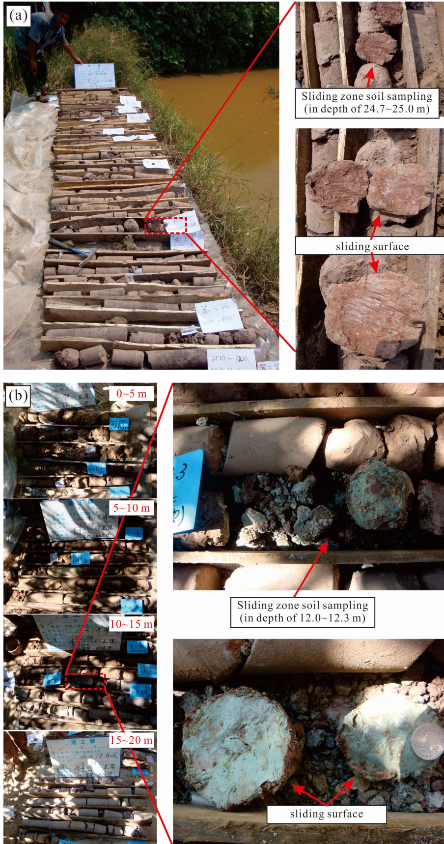
Fig. 5. Sampling of sliding zone soil from the Tangjiao landslide: (a) borehole ZK1-111 and (b) borehole ZK1-139. Note: the locations of the two boreholes are shown in Fig. 2a.
