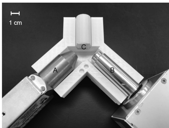
Fig. 1. Experimental setup for XRF measurement of stainless steels. (A) X-ray tube. (B) Detector. (C) sample. The holder of devices was made by using a 3D printer. The material of the holder was polylactic acid. The incident and takeoff angles were 45 degrees. The distance among the X-ray tube, sample, and the detector were 2 cm.
