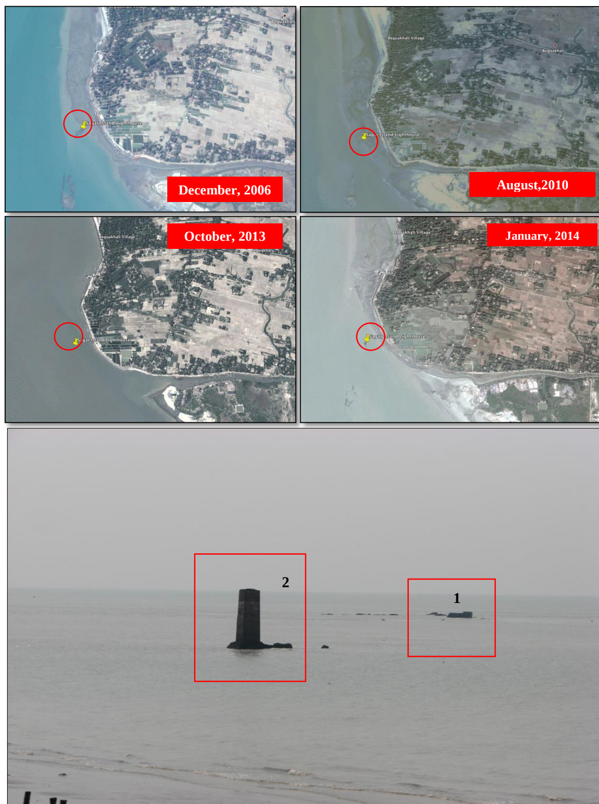
Figure 1.6. (Top) Recent Satellite Images of the Lighthouse in Sagar Islands, gradually being swollen by the rising sea. The latest images (2013 and 2014) also show the existence of newly constructed sea-dyke to prevent further inundation. (Bottom) The photograph depicting the same, the old remains of the lighthouse is visible through the sea. Source: Google Earth (Top) and Author, 2013
