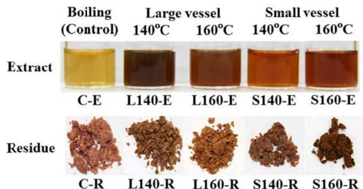
Fig. 5-2. Appearance of the liquid extracts and solid residues obtained using the large and small vessels at 140 and 160 °C. Labels L and S and values 140 and 160 are the same as in Fig. 5-1. E and R indicate the extract and residue, respectively. C-E and C-R indicate the extract and residue, respectively, obtained from the boiling treatment (control).
