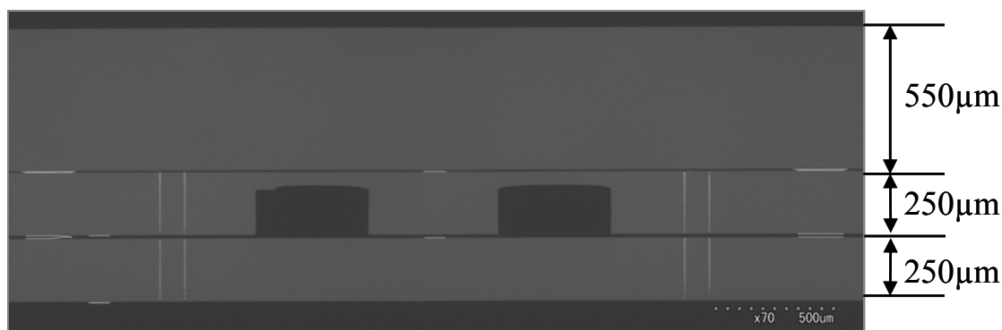
Fig.4.27 Cross-sectional view of three bonded layers including an MEMS layer having a bridge structure; MEMS layer is a piezoresistive 3-axis accelerometer.
