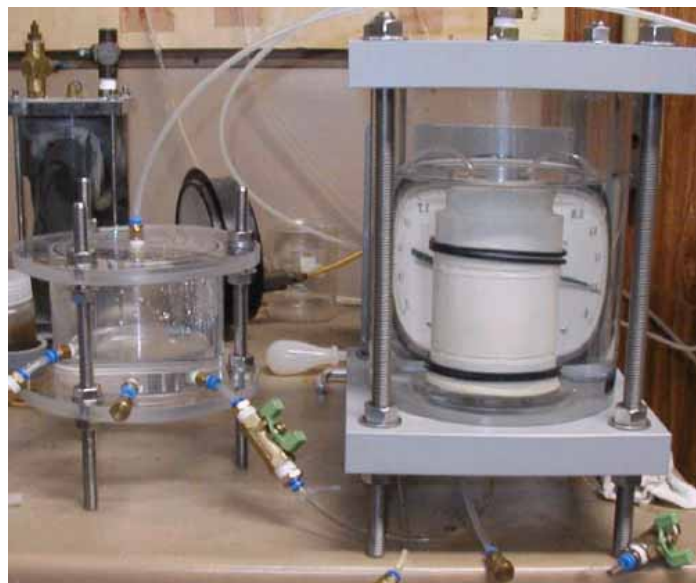
Figure 3.11 Laboratory flexible-wall column testing.
