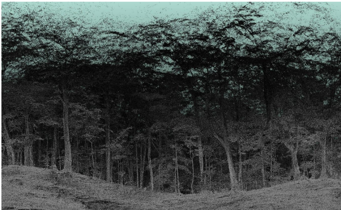
Fig. 5.2 A vertical profile of BLK2GO mobile Terrestrial Laser Scanner (TLS) data which can effectively scan under-canopy trees. An example from the Tsushima evergreen broadleaf forest in southern Japan.
