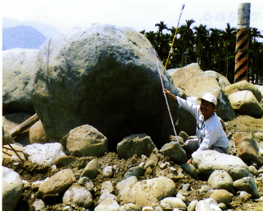
Photo 5 Big boulders and sediments flooded and deposited on the landside area at Mujiliao district due to bank breach of the Tungpurui Chi
