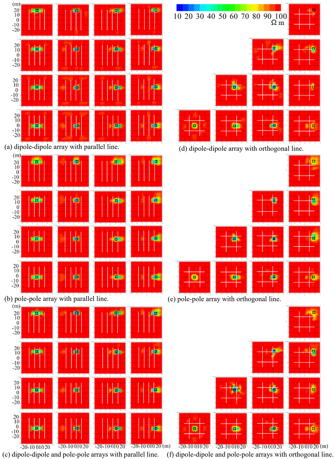
Figure 4.4 A resistivity slice at depth of 4 m reconstructed from 3D inversion of synthetic data obtained along four parallel lines (a, b and c) and four orthogonal lines (d, e and f). The square black box shows the location of the conductive body in the half-space.
