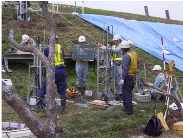
Fig. 1 Vertical measurement by NSWS testing machine
