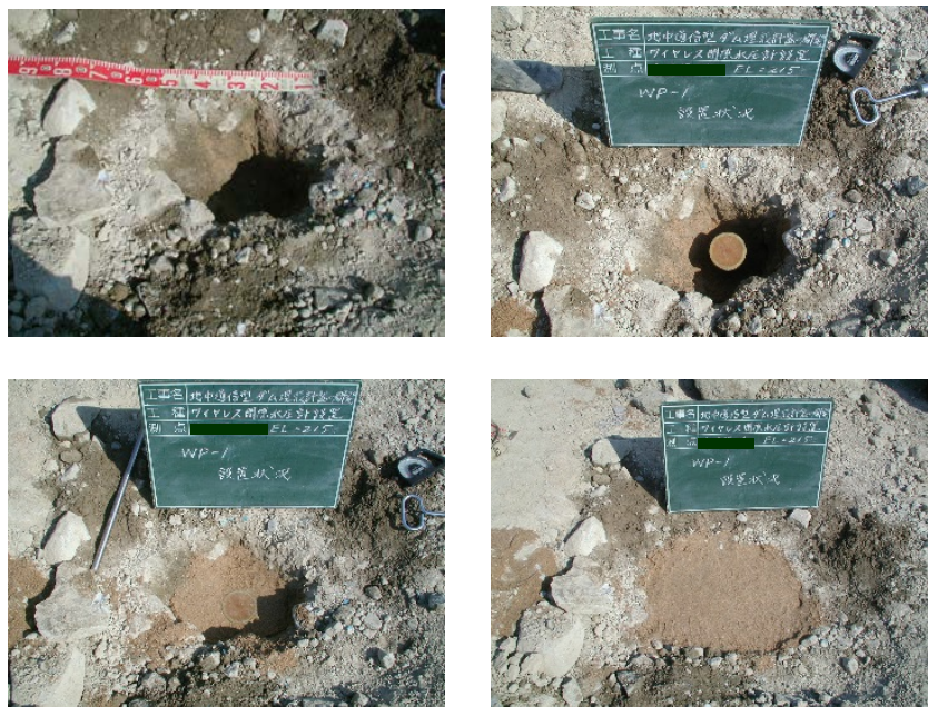
Figure 3.11 Outline of WPT installation in semi-pervious zone
