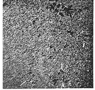
Photo 17. Modified with 0.1% Na \times 100
