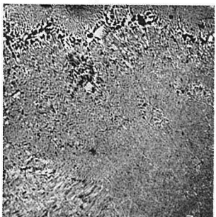
Photo 10. Modified with 0.3% Al \times 100
