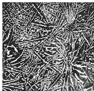
Photo 3. Modified with 0.3% Na \times 100
