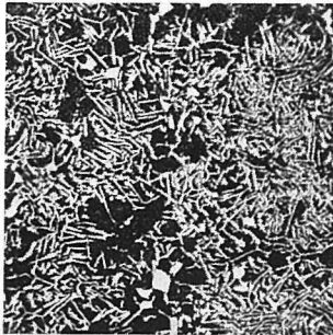
Photo 21. Modified with 0.15% As \times 100
