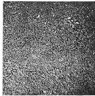
Photo 19. Modified with 0.1% Ca \times 100
