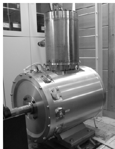
Fig. 5 Photograph of the 20 kW-class HTS-ISM designed for automobile applications 25) .
