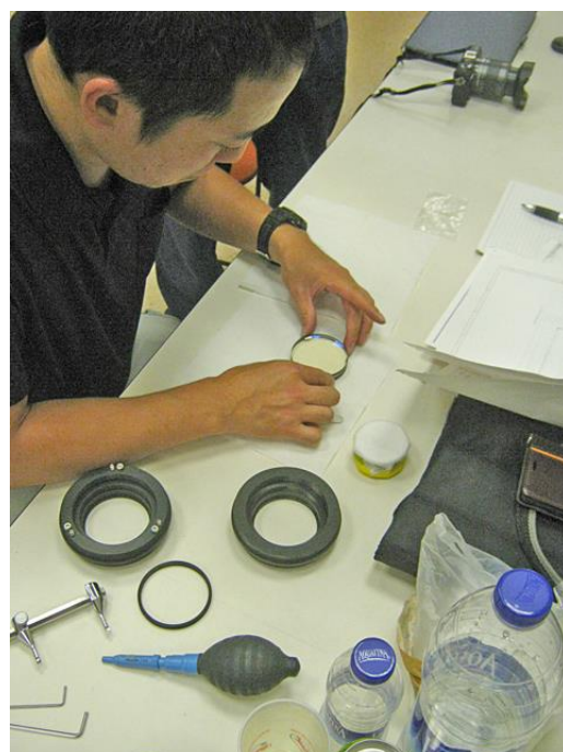
Photo 5: Adjustment of the alignment of objective lenses (Oct 2015)
