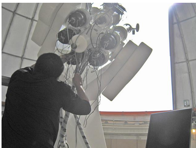
Photo 6: Adjustment of observational wavelengths of optical filters (Oct 2015)
