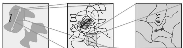
Figure 8 Hierarchical structure of SBR rubber swollen by d-hexane/hexane.
