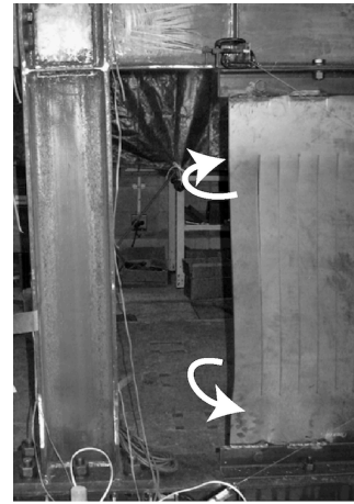
(b) Exterior flexural links
