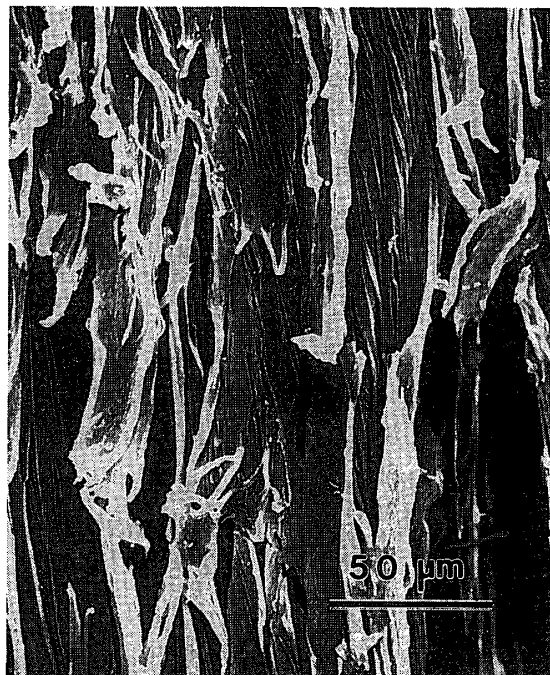
Fig 1.30. Formaldehyde-treated LVL after exposure to artificial weathering for 720 hrs, showing diagonal fissures following the microfibril angle of the S 2 layers.
