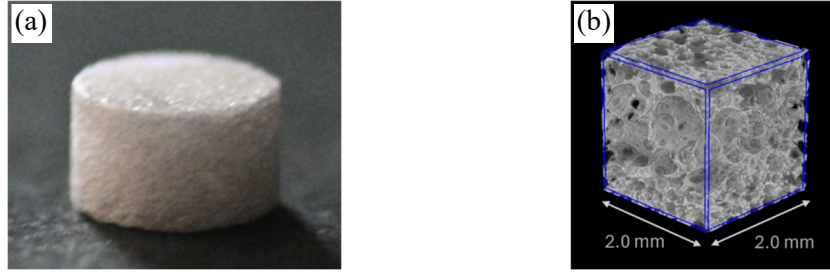
FIGURE 1 (a) Cylindrical pullulan foam obtained from a mixture of c_w = 0.20 at 200 °C and (b) 3D-image of its inner cellular structure.
