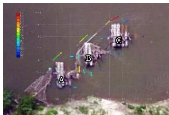
Fig. 16 Flow patterns (220 m 3 /s)
