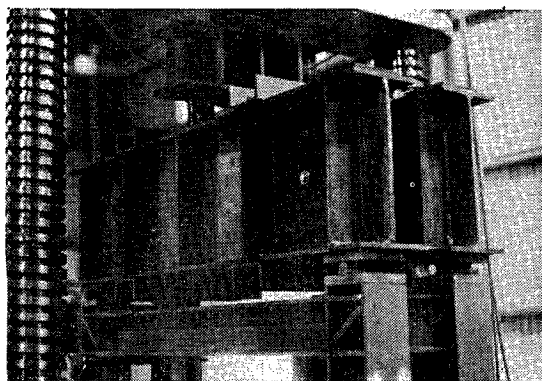
Photo. 4 Vertical loading system
