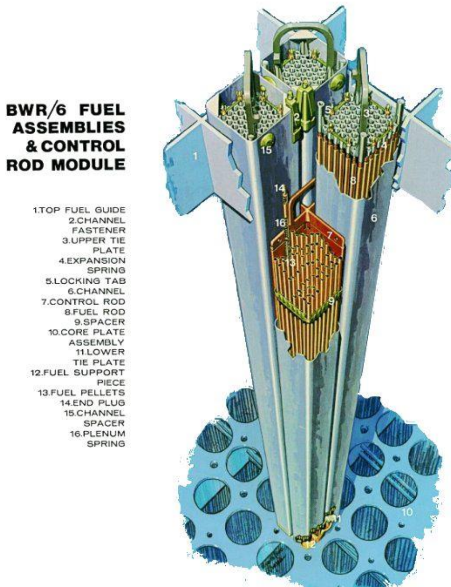
Figure 1-2 Schematic view of BWR fuel assembly ( www.world-nuclear.org )
