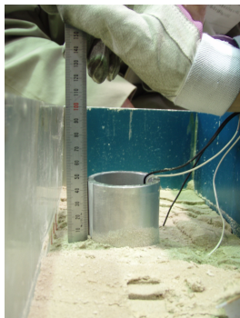
Fig. 11 Uplifted manhole (Case 5)
