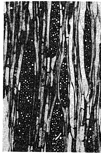
Photo. 5. BUNA( t , 55 x), transversal penetration. Not so permeable to radial direction in spite of the existence of multiseriate rays, because their consisting ray cells were filled with much contents.
