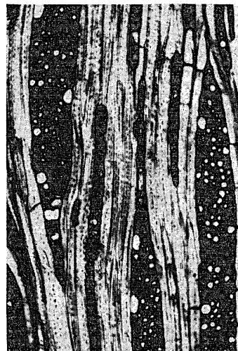
Photo. 6. Apitong( t , 55x),transversal penetration. Similar as in the case of BUNA shown in the explanation of Photo. 5.
