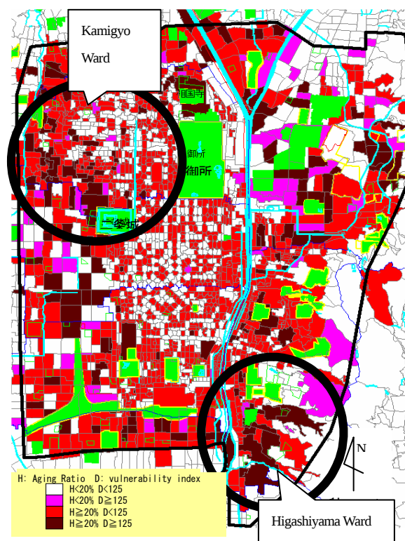
Fig.5 Distribution of weak areas against earthquake
