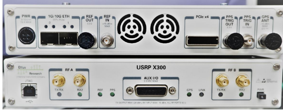
FIGURE 3.1: Front and rear interface of USRP X300
