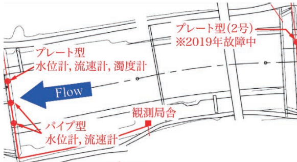
Fig. 2 Observation equipment at the Okawara measuring station
