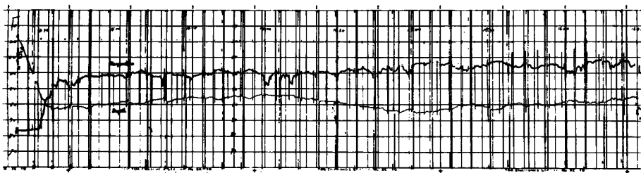
Fig. 7 An example of record of the vertical displacement of the INBF and its surrounding water temperature obtained from the underwater acoustic signals which were send out from the INBF.
