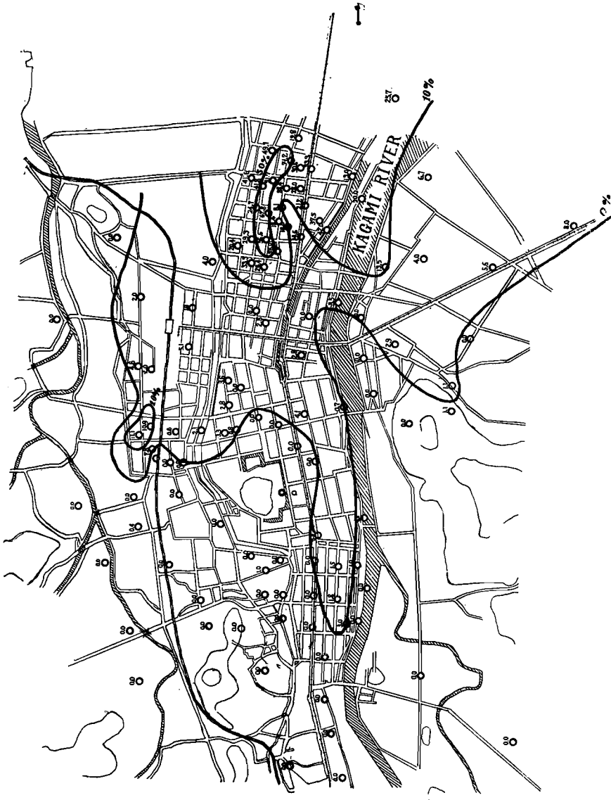
Fig. 23 The rate of complete damage at Kōchi.
