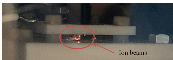
Fig. 11. Image of ion beams when supplying from back side of emitter chip.
