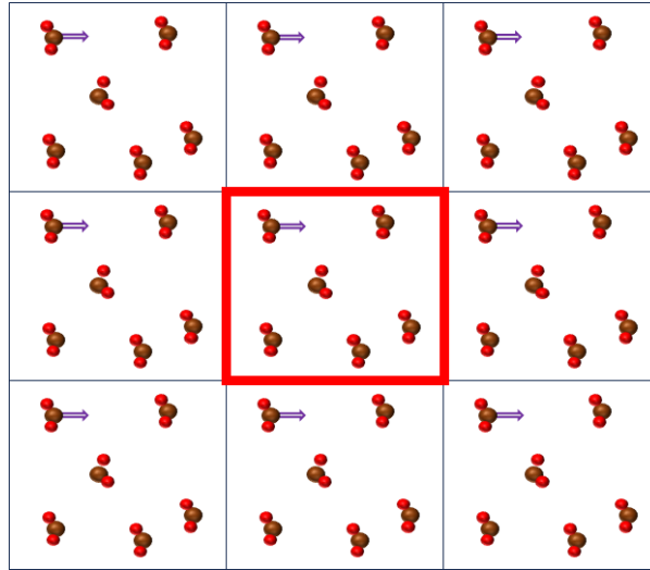
Figure 2. 2. The schematic diagram of Periodic Boundary Condition (PBC)
