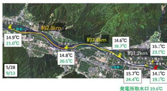
Fig. 5 Observed data (downstream of Power plant)
